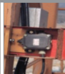
과부하방지장치(Over Load Limiter)
